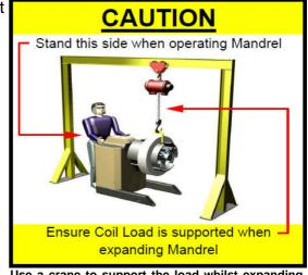
Use a crane to support the load whilst expanding the mandrel
