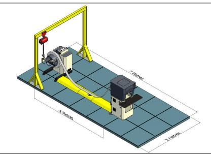
Typical AEM Decoiler Installation with a Unicore machine
