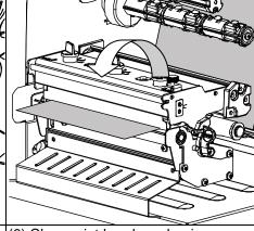
6) Close print head mechanism, making sure the latches are engaged properly.
