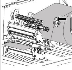
(4) Pull the leading edge of the label forward through the media guide bar past media sensor, and place the leading edge onto the platen roller. Adjust the rear label guide to fit the label width.
