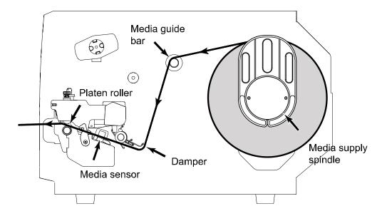
(7) Using the front display panel, set media sensor type and calibrate the selected sensor. (See "Media Sensor Calibration" on facing page.)
