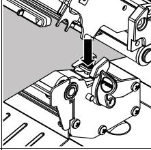
(5) Press and hold the front label guide to adjust it to fit the label
