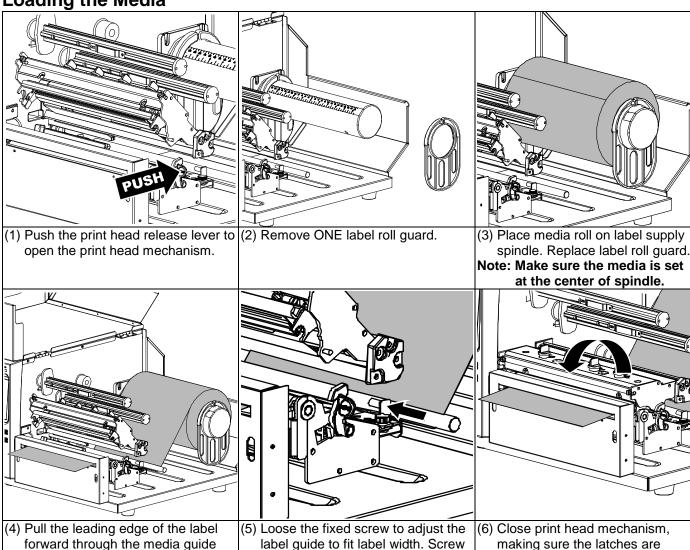
bar past media sensor, and place the leading edge onto the platen roller.
