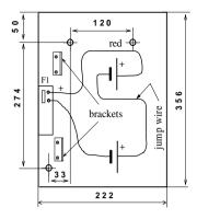
cable to the wires going out of the power supply board (observing polarity). Ensure the temperature of the F1 fuse doesn't essentially exceed the room temperature. If the temperature of the fuse is higher, inspect once more the batteries for proper connection. Close the box cover and tighten up two side screws.
