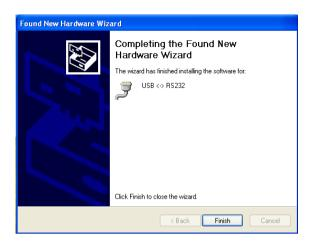
Now the S2000-USB driver has been installed. READY indicator on the S2000-USB face plate should be lit steady. After driver setup, Ports (COM&LPT) of the Device Manager will include the 'USB <-> RS-232 (COM x)' entry where 'x' is the number of the virtual COM port:
