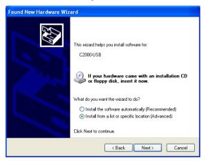
Next, in the window for selecting driver location select the options as shown in Figure below and specify the path to the S2000-USB driver. Click Next:
