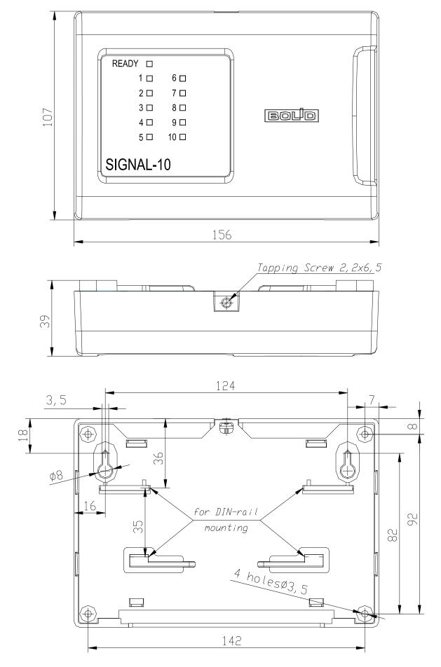
Figure 2. Signal-10 Overall and Mounting Dimensions
